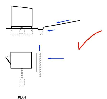
Install a land-drain to prevent flooding of soakaway area.
